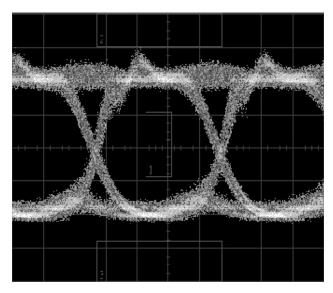
Figure 7. ADN2847 Unfiltered 2.5 Gbps Optical Eye. Average Power = -3 dBm, Extinction Ratio = 10 dB. Eye Obtained Using a Mitsubishi FU-445-SDF.
