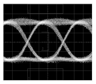
Figure 8. ADN2847 Filtered 2.5 Gbps Optical Eye. Average Power = –3 dBm, Extinction Ratio = 10 dB. Eye Obtained Using a Mitsubishi FU-445-SDF.
